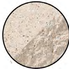
MASONRY 8"X16" BLOCK IN ROUGH GRADIENT BOTTOM TO TOP OF SPLIT FACE TO SMOOTH FACE COLOR: PARCHMENT
