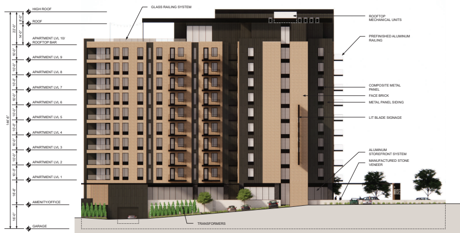
SOUTH ELEVATION SCALE: 1" = 20'-0"
