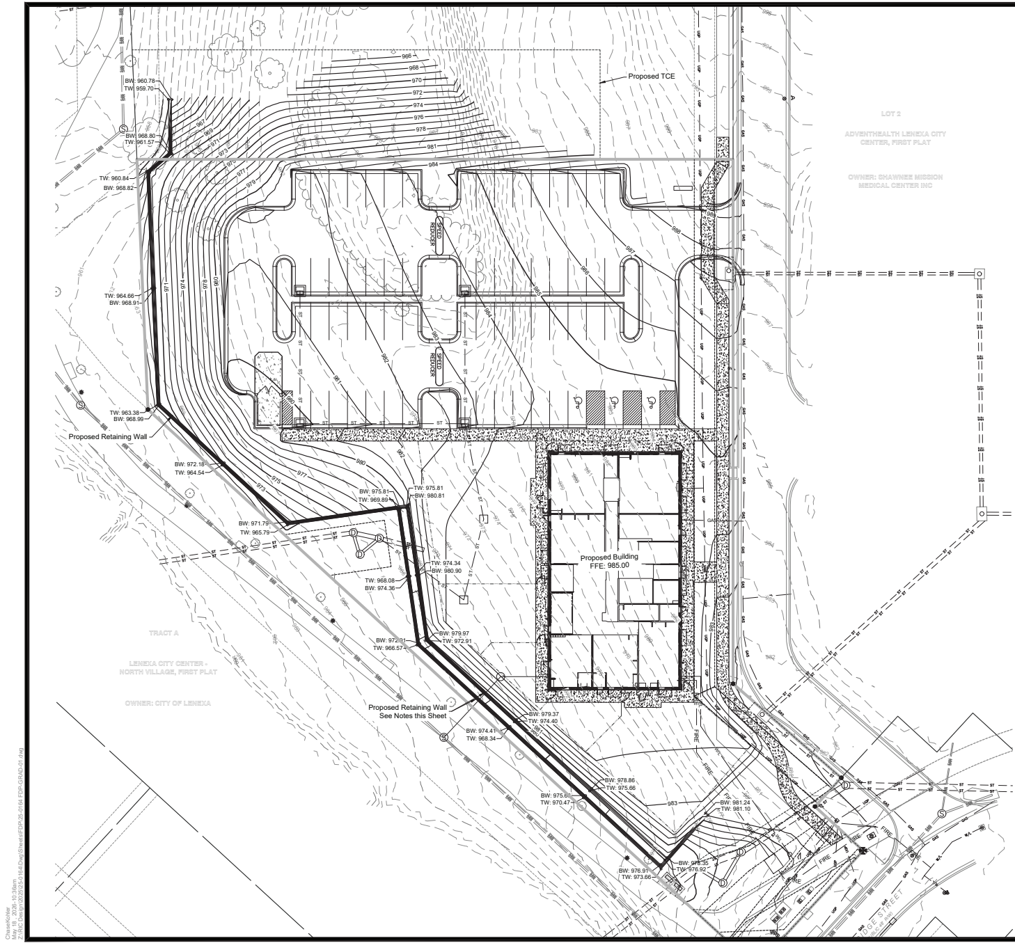
Wall Design Intent: Belgard Diamond Pro Meriam Blend Straight Face Retaining Wall or Approved Equal. Final block manufacture and color to be reviewed and approved at permit level.
