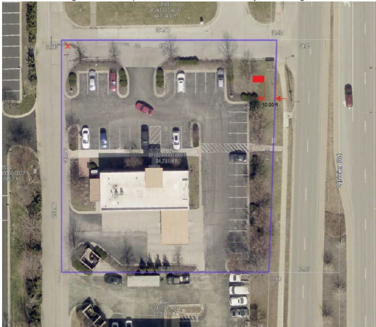
Exhibit 4: Aerial view demonstrating the setback of the proposed monument sign, meeting the UDC requirement.
