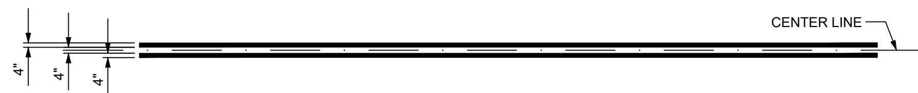
TYPICAL 4" SOLID YELLOW DOUBLE LINE DETAIL
