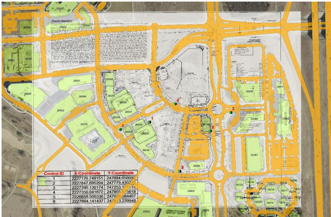
Figure 3. An example of a GIS Site Plan sheet georeferenced into a GIS system.
