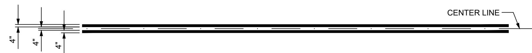
TYPICAL 4" SOLID YELLOW DOUBLE LINE DETAIL
